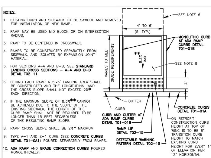
11. ALL RAMPS IN AREAS ZONED CITY CENTER OR WHERE THE HERITAGE SIDEWALK IS CONSTRUCTED ARE REQUIRED TO BE CONSTRUCTED WITH BRICK UNIT PAVERS, SEE BRICK UNIT PAVER PATTERN TO2-16 FOR BRICK LAYOUTS.
