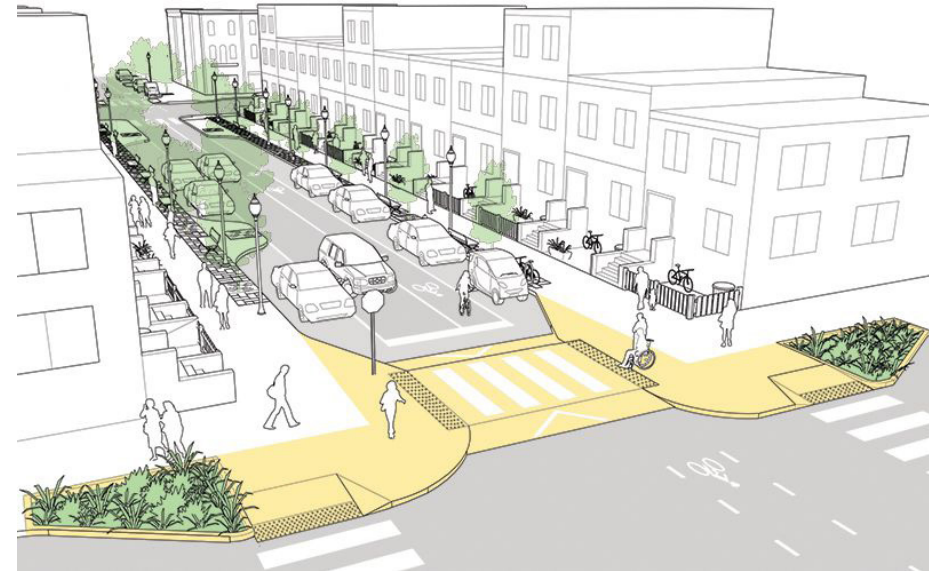
Figure 17. Raised crosswalk concept for 39th Street
