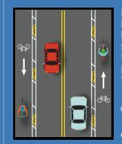
Protected bike lanes include bike lanes by the curbs, with buffer areas on the driving lane sides. The buffers include vertical devices that keep people driving from entering the bike lanes.
