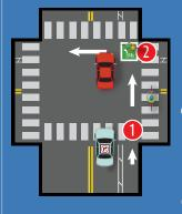
Two-stage left turn boxes are designed to give bicyclists a safe way to turn left through an intersection
