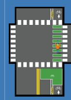
Bike lane extensions are designed to provide a visable area of travel through an intersection
