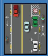
Parking-protected bike lanes include bike lanes by the curbs, with buffer areas on the driving lane sides. There is a parking lane between the bike lane buffer and the driving lane on one or more sides of the street.
