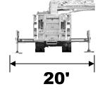
NOTE: A width of up to 30' may be required where it is determined that additional apparatus or pedestrian access width could be necessary.
