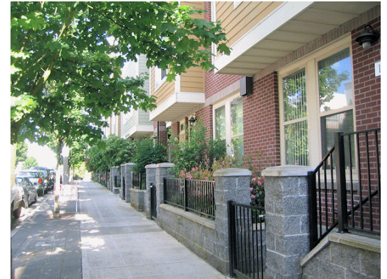
Figure 11. A good example of a departure with a reduced setback. The low fence and landscaping provide an effective transition between the sidewalk and street.
