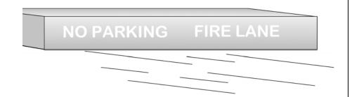
Stencil placement is 20 feet on center and at changes in direction where the lettering may not be visible from a vehicle.
