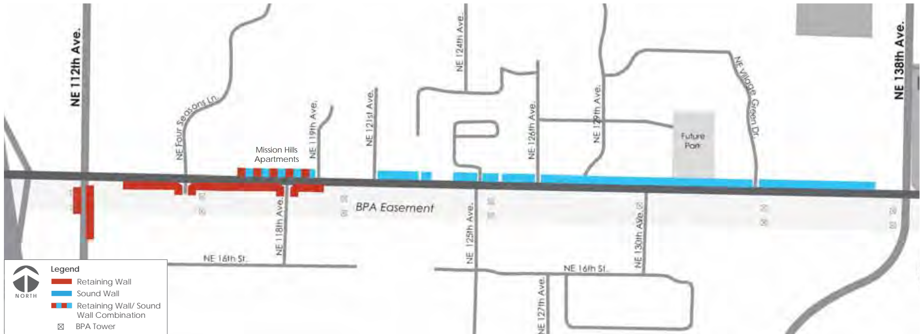
NE 112th Avenue to NE 138th Avenue Sound and Retaining Walls
