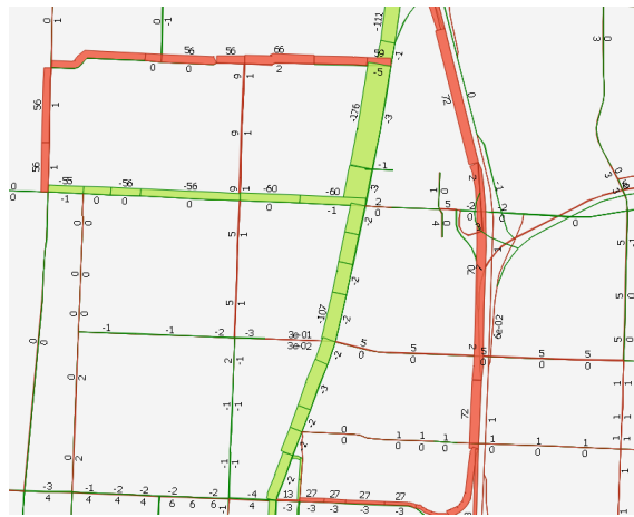
Figure 2. Volume diversion with Main Street roadway reconfiguration for the year 2040 AM peak period
