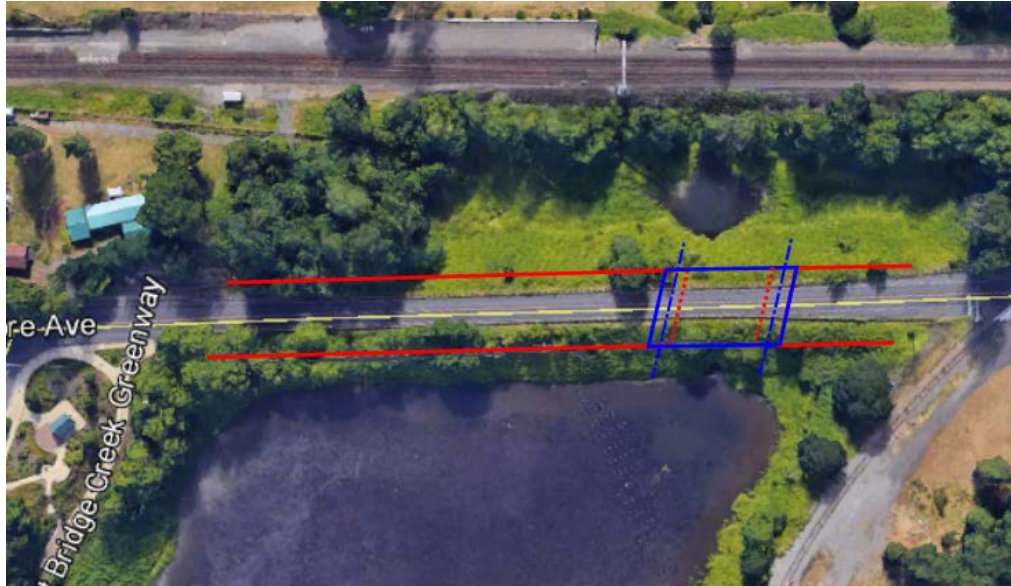
Figure 12. Burnt Bridge Creek embankment widening with bridge
