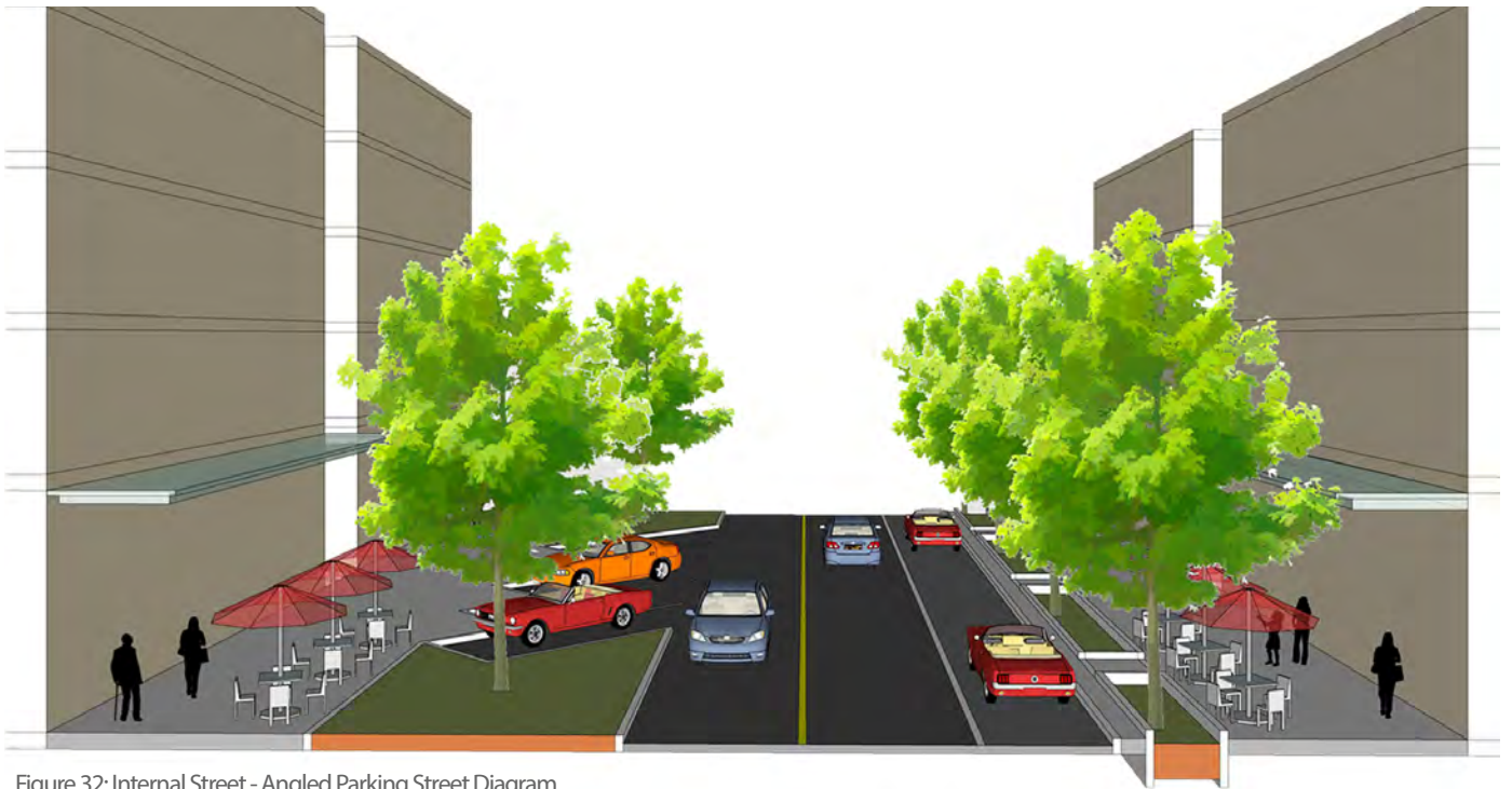
Figure 32: Internal Street - Angled Parking Street Diagram
