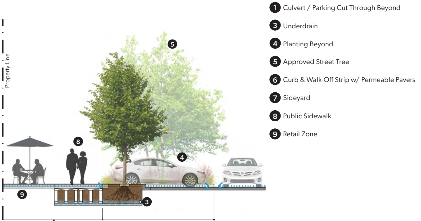
Figure 42: Silva Cell with Tree Grate Diagram
