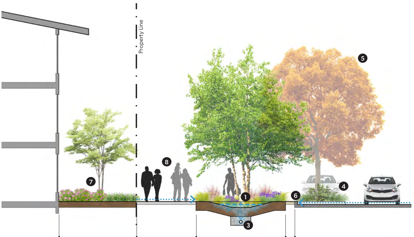
Figure 43: Bioretention Swale Diagram
