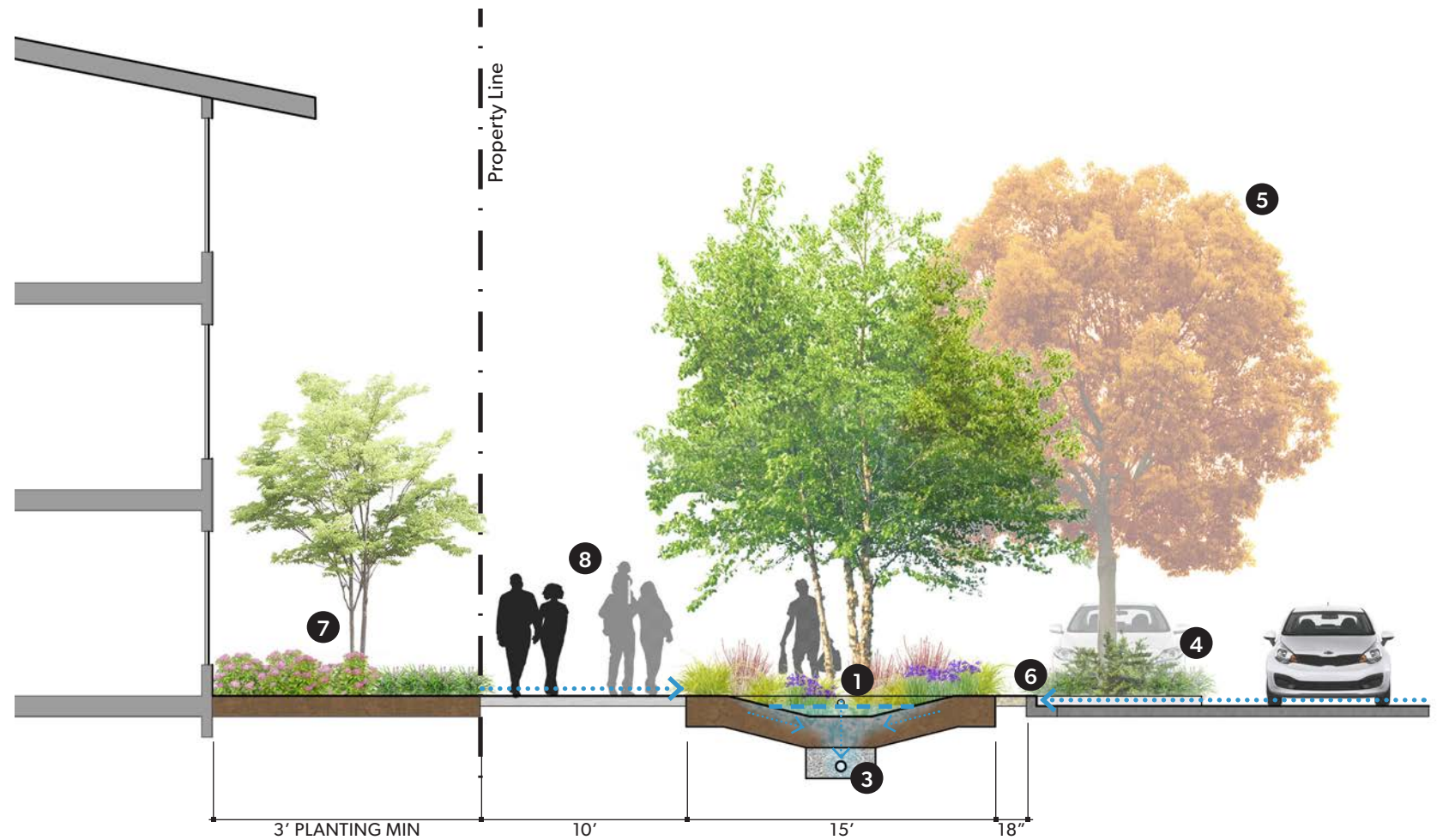
Figure 5: Bioretention Swale SCALE: 1/8" = 1'
