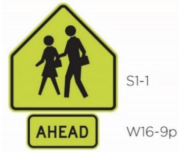
Figure 6 Crossing Warning Assembly
