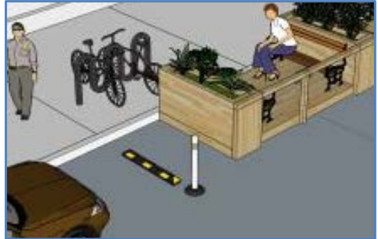
Wheel stop and reflective delineator post
