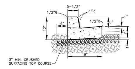
5 PROPOSED TYPE A-1 CURB AND GUTTER (FOR ADDITIONAL INFORMATION SEE CONCRETE CURB DETAIL TO1-01A)
