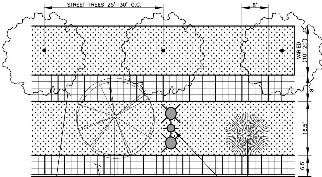
8' MIN. WIDE CONCRETE SIDEWALK, SEE **SIDEWALK DETAIL T02-01A**
