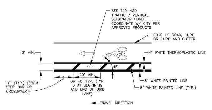
BIKE LANE BUFFER ZONE AREA MARKING WITH TRAFFIC / VERTICAL SEPARATOR CURB
