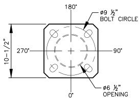
DO NOT USE TO SET ANCHOR BOLTS CONTACT CUSTOMER SERVICE FOR TEMPLATE
