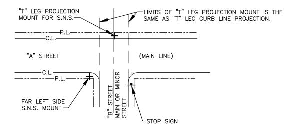
WHEN A "MAIN LINE" STREET AND A MINOR "T" LEG STREET OR TWO "MAIN LINE" STREETS INTERSECT AT A "T" INTERSECTION, SIGNS SHALL BE MOUNTED INSIDE THE CURB LINE ON BOTH SIDES OF THE THROUGH STREET. ONE SET OF SIGNS SHALL BE ERECTED "FAR LEFT SIDE" AT THE "T" LEG. THE OTHER SET OF SIGNS SHALL BE MOUNTED AS CLOSE AS POSSIBLE TO THE "T" LEG CENTER LINE PROJECTION. FOR ADDITIONAL SIGN INFORMATION, SEE GROUND MOUNTED STREET NAME SIGN DETAIL, T29-01.
