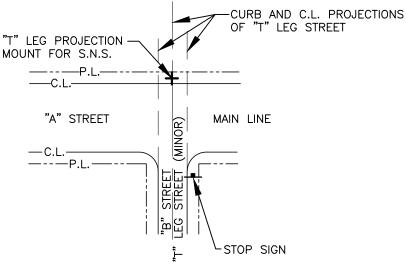
WHEN TWO MINOR STREETS INTERSECT AT A "T" INTERSECTION, SIGNS WILL BE MOUNTED INSIDE THE CURB LINE OF THE THROUGH STREET ON THE SIDE OPPOSITE THE "T" LEG AND WITHIN THE CURB LINE PROJECTIONS OF THE "T" LEG STREET. SIGNS WILL BE MOUNTED AS CLOSE AS POSSIBLE TO THE "T" LEG CENTER LINE PROJECTION. FOR ADDITIONAL SIGN INFORMATION SEE GROUND MOUNTED STREET NAME SIGN DETAIL, T29—01.
