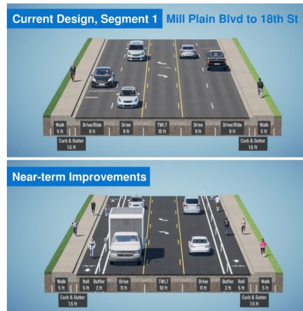
Figure 2: 112 th Avenue proposed near-term improvements between SE McGillivray Blvd and NE 18 th Street
