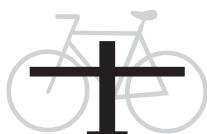
These racks are intended to capture a bike's frame and both wheels with a pivoting arm. In practice, they accommodate only limited bike types and have moving parts that create unneeded complications.
